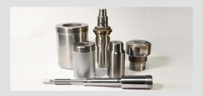
Joining of tungsten carbide to a metal component is used to address manufacturing issues regarding fabrication, assembly and cost.
