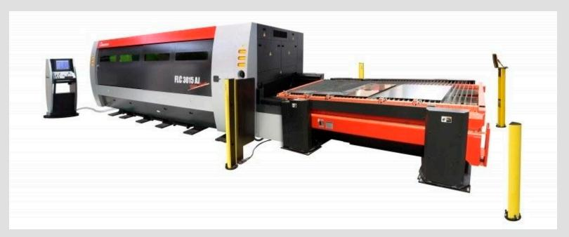
High Speed, 2 kilowatt fiber laser system with capability to cut up to 7/8" thick mild steel or 3/8" thick stainless steel. The laser system provides an additional option for prototype and development parts as well as a cost efficient option for lower volume production requirements.
